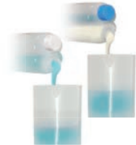
Pour TechnoGelGum into the provided beaker in a 1:1 ratio.
