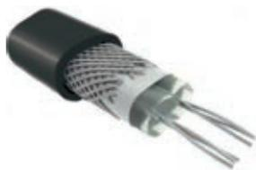
**Power:** 20 W/m**Power supply:** 230 V ~ 50/60 Hz**Heating cable dimensions:** ~ 5 x 7 mm**Min. installation temperature:** + 5°C**Max. working temperature:** + 80°C**Cold cable (power supply):**length 4 meters - 3 x 1,0 mm<sup>2</sup> or 3 x 1,5 mm<sup>2</sup>**Heating cable type:**
