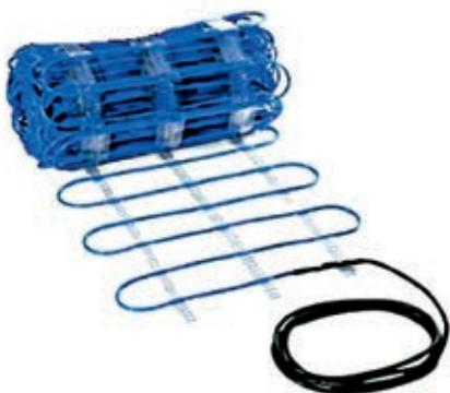
**CHARACTERISTICS****Mat specific power:** 300 W/m<sup>2</sup>**Power supply:** 230 V ~ 50/60 Hz**Mat thickness:** 7,5 mm**Min. installation temperature:** + 5°C**Max. working temperature:** + 80°C**Cold cable (supply):**length 4 meters - 3 x 1,5 mm<sup>2</sup> or 3x2,5 mm<sup>2</sup>**Heating cable type:**
