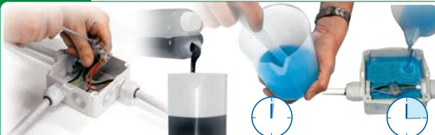
You can use the Magic Power gel supplied in the two-component bottle in a 1:1 ratio by simply pouring it after mixing into the box supplied in the kit, to protect and seal internal connections. The gel cross links in just 15 minutes, but the box can be energised immediately.
